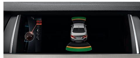
**Rear-view Camera** shows on the Control Display the area behind your vehicle. Guidelines indicate if your vehicle can fit in a parking space, and display parking turn angles. The Rear-view Camera is activated by engaging reverse gear.
