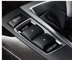
**Driving Dynamics Control** adjusts driving characteristics by pressing a button to select one of five settings. Choosing COMFORT, COMFORT+, SPORT, SPORT+ or ECO PRO mode adjusts the engine-throttle response, shift characteristics and power-steering assist. Another button disengages the traction control feature when driving on sand, gravel, or deep or packed snow.
