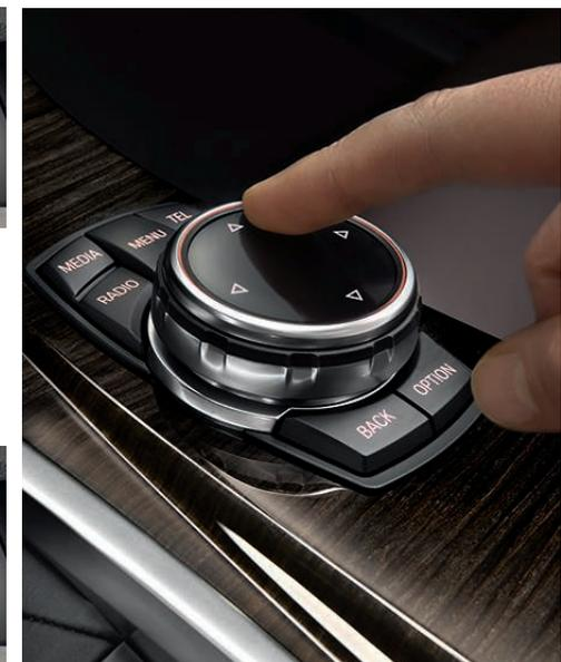
**iDrive touchpad Controller** allows intuitive, convenient operation of the iDrive system. Using the Controller-integrated touchpad, you can enter destination addresses for the Navigation system by using your own handwriting, while the input is conveniently shown in the Control Display.
