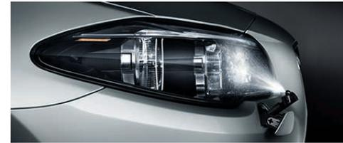
The **headlight washing system** maximizes illumination of the road ahead in all weather. When the windshield washer function is activated, headlights are also automatically cleaned.
