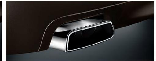
**Tailpipes.** The 550i and 550i xDrive display two rhombus-shape tailpipes covered with a chrome frame – one on the left, one on the right.
