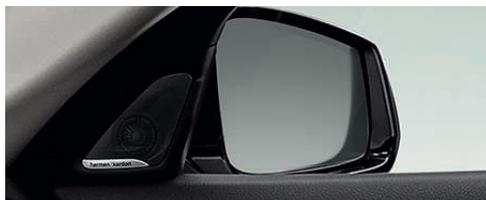
**Harman Kardon® Surround Sound system** is a 16-speaker system with 600-watt digital amplifier and Dirac signal processing that outputs reproduction of the surround information contained in the stereo signal in a nine-channel format, as well as 5.1 surround sound from a DVD source. The system also compensates for driving noise in smooth steps with speed-dependent equalizing.
